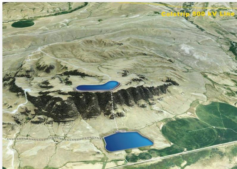
We want to take run-of-river hydro and wind at night, and regulate that. We pump at night. During the day, we go to gen mode and still handle the integration of wind outbound east of the Colstrip system to replace coal capacity. This facility is in a strategic location to get more value out of the facilities in the ground,” he said.
